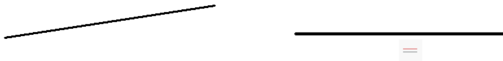
Left: Line drawn at an arbitrary angle; right: Line snapped flat by horizontal constraint
