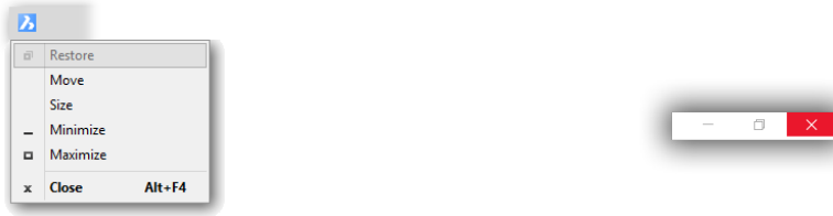
Left: Control menu at left end of title bar; right: equivalent control buttons at right end of title bar.
