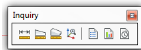
From left to right: Distance, Area, Mass Properties, ID Coordinates | List Entity Data, Drawing Status, Time Variables
