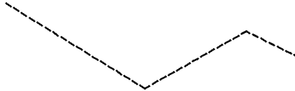
Drawing line segments with hidden linetype automatically applied
